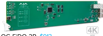
OG-FiDO-2R $913 openGear 2-Channel Single Mode LC Fiber to 3G-SDI Receiver
