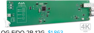
OG-FiDO-2R-12G $1,863 openGear 2-Channel Single Mode LC Fiber to 12G-SDI Receiver
